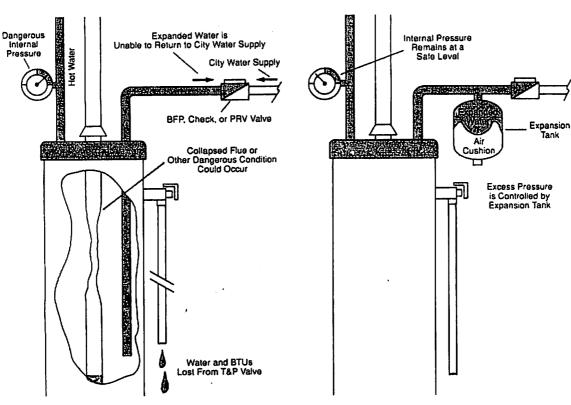
The Problem: In the "Good Old Days", before the advent of cross-connection control, expanded water which exceeded the capacity of the water heater flowed back to the City main where it was easily dissipated. But today, with the backflow preventers, water meters with check valves, and/or pressure reducing valves without bypass being installed, expanded water from a water heater cannot return to the City supply. It is now a closed system, and the expanded water has no place to go.
